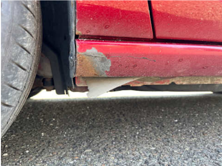
Schweller links (Lackschaden, Rost)
