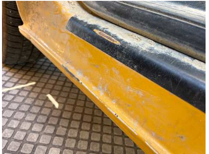
Schweller links (Lackschaden, Rost)
