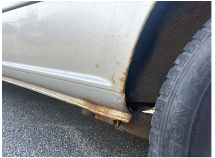
Schweller links (Lackschaden, Rost)
