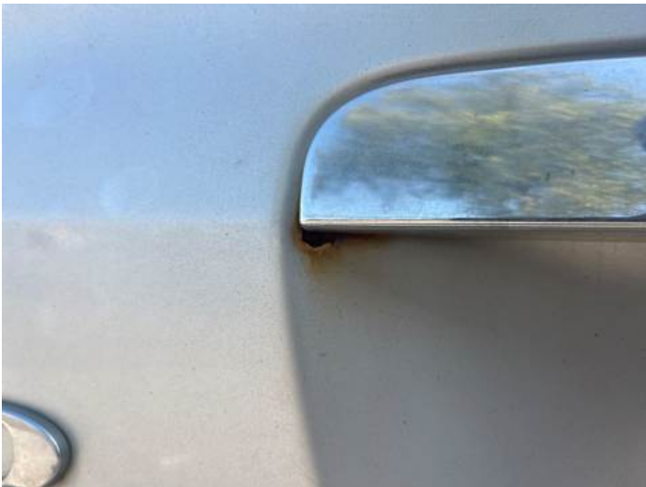
Heckklappe (Lackschaden, Rost)
