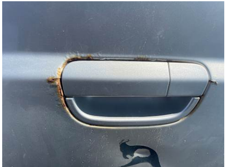
Heckklappe (Lackschaden, Rost)
