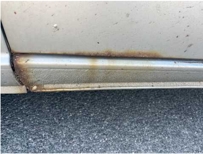
Schweller links (Lackschaden, Rost)
