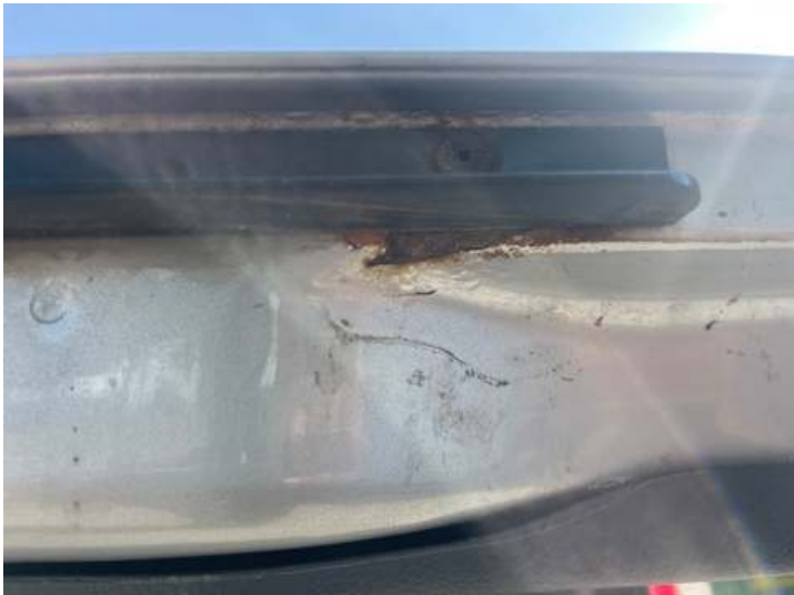
Heckklappe (Lackschaden, Rost)
