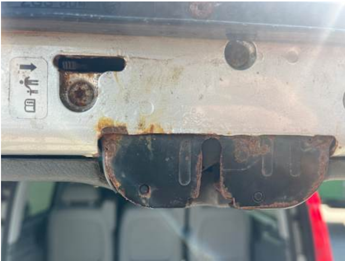
Heckklappe (Lackschaden, Rost)
