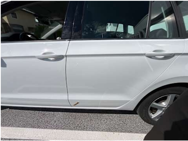
Türe hinten links (Lackschaden, Rost)
