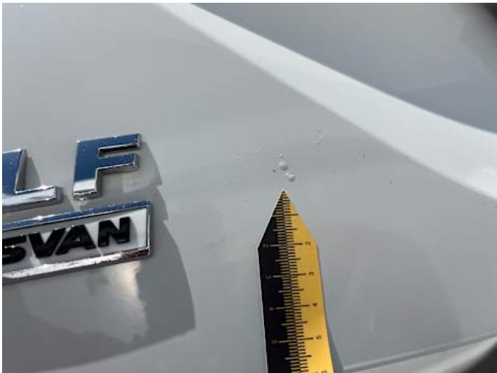
Heckklappe (Lackschaden, Rost)
