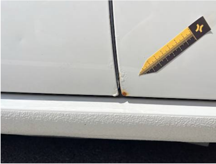
Türe hinten links (Lackschaden, Rost)
