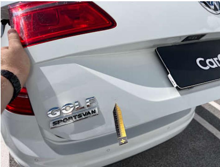
Heckklappe (Lackschaden, Rost)
