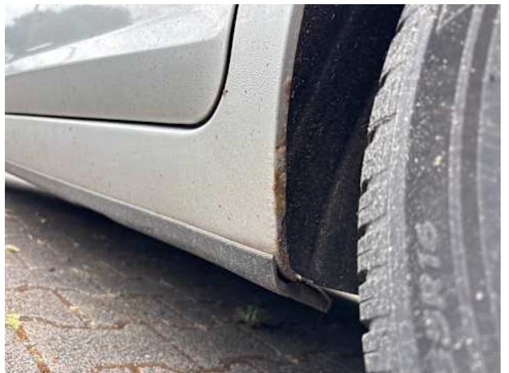
Schweller links (Lackschaden, Rost)
