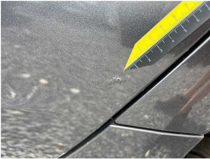
Türe hinten links (Lackschaden, Rost)
