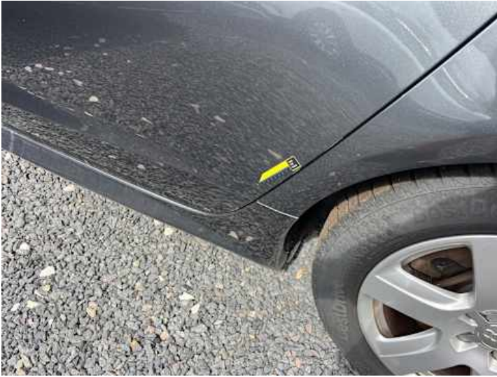
Türe hinten links (Lackschaden, Rost)
