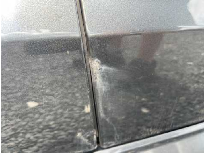
Türe hinten links (Lackschaden, Rost)
