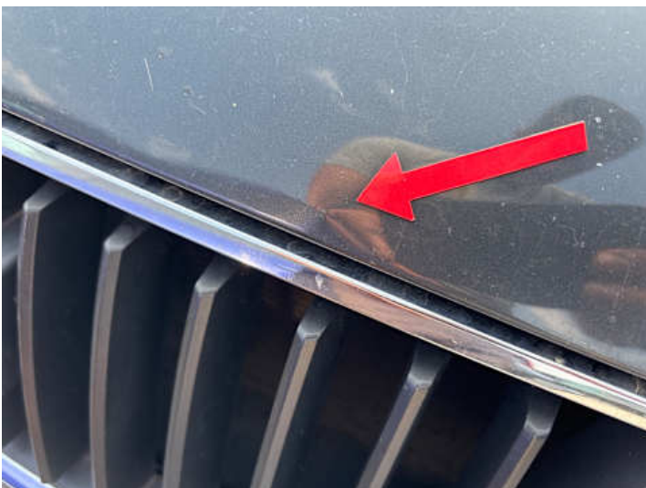
Motorhaube (Delle, Rost)
