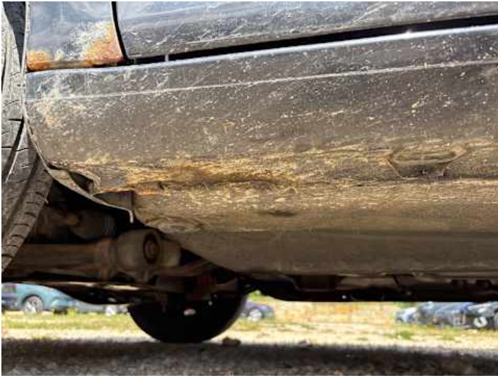
Schweller links (Lackschaden, Rost)
