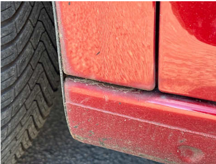
Schweller links (Lackschaden, Rost)
