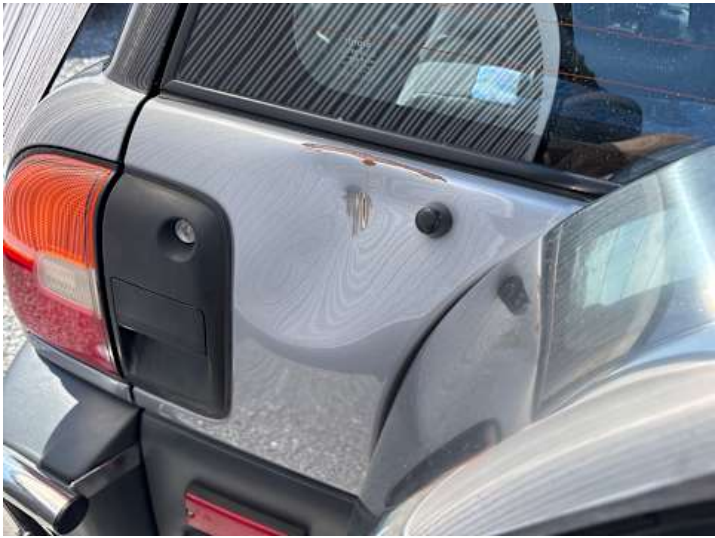
Heckklappe (Lackschaden, Delle, Rost)
