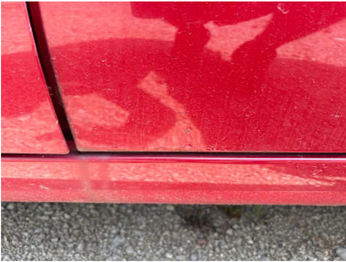
Türe hinten links (Lackschaden, Rost)
