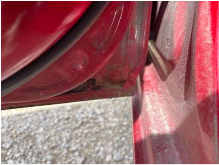
Türe hinten links (Lackschaden, Rost)
