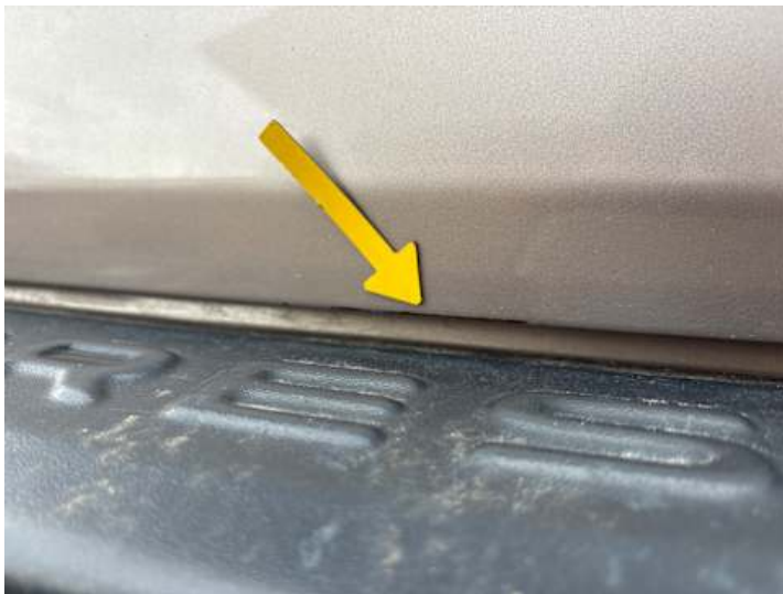
Heckklappe (Lackschaden, Rost)
