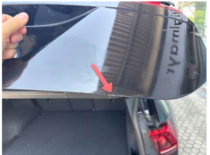
Heckklappe (Lackschaden, Rost)
