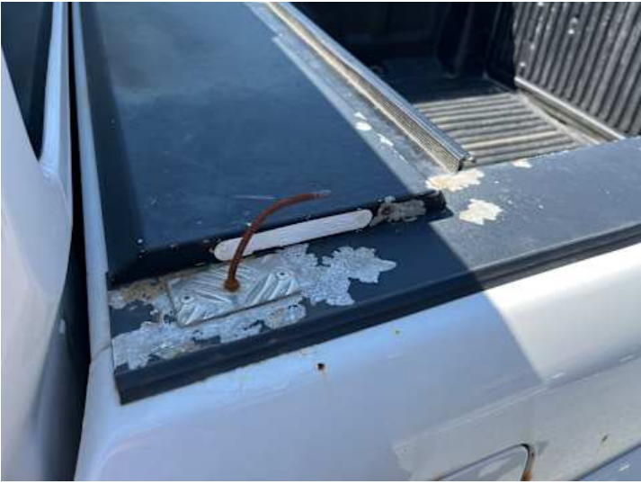
Heckklappe (Lackschaden, Rost)
