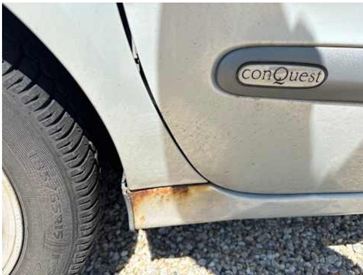
Schweller links (Lackschaden, Rost)
