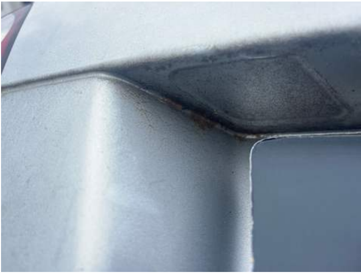
Heckklappe (Lackschaden, Rost)
