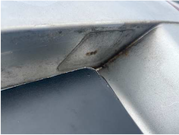
Heckklappe (Lackschaden, Rost)
