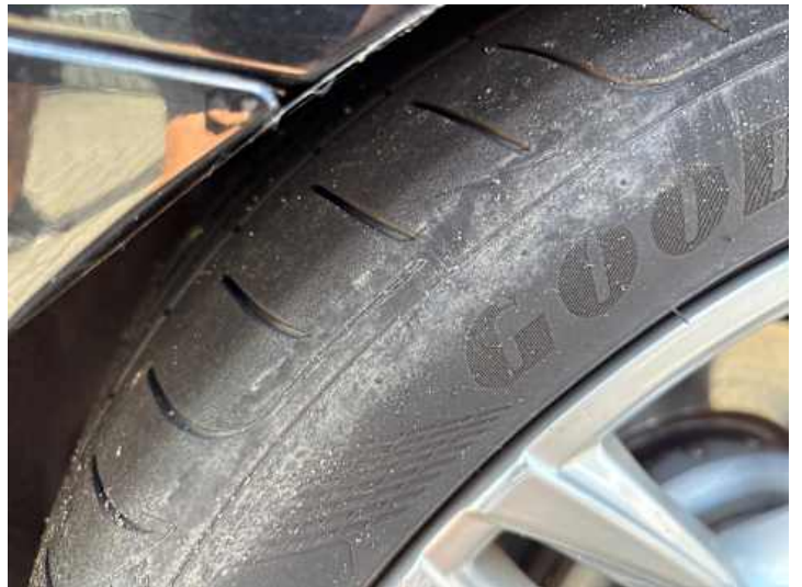
Rad (Kerben, vehicle.damage-label.porous)
