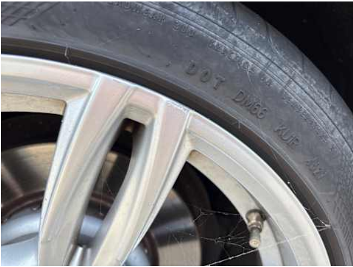
Rad (Kerben, vehicle.damage-label.porous)
