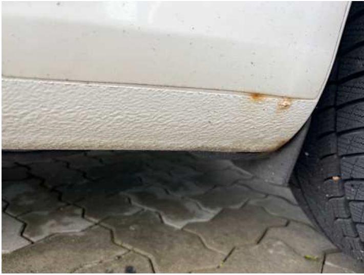
Schweller links (Lackschaden, Rost)
