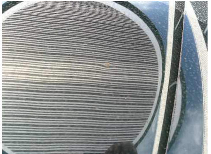
Motorhaube (Delle, Rost)
