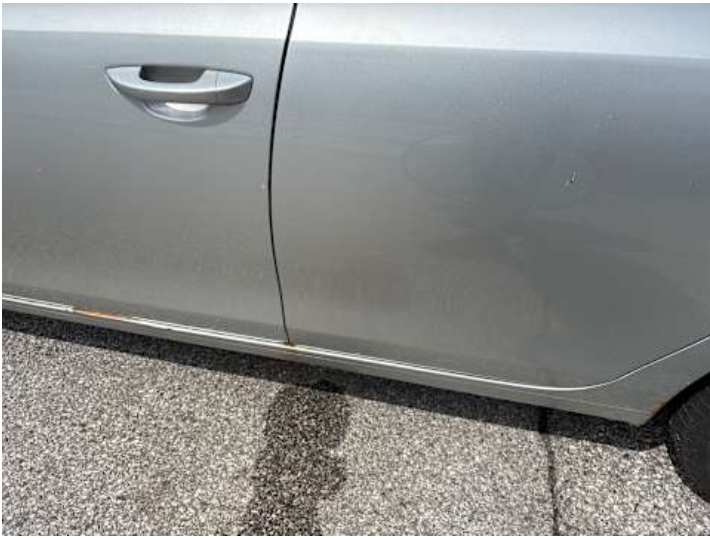
Türe hinten links (Lackschaden, Rost)
