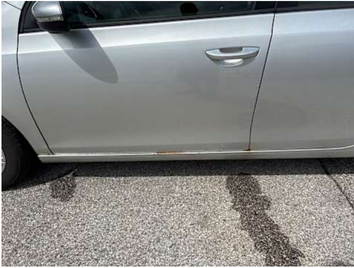
Schweller links (Lackschaden, Rost)
