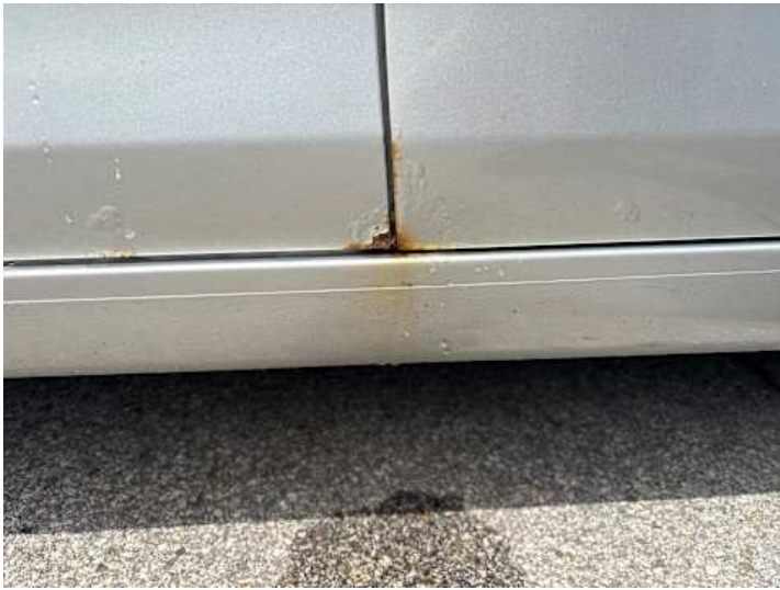
Türe hinten links (Lackschaden, Rost)
