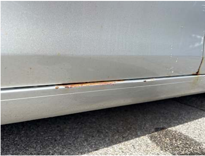
Schweller links (Lackschaden, Rost)
