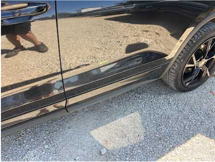
Türe hinten links (Lackschaden, Rost)
