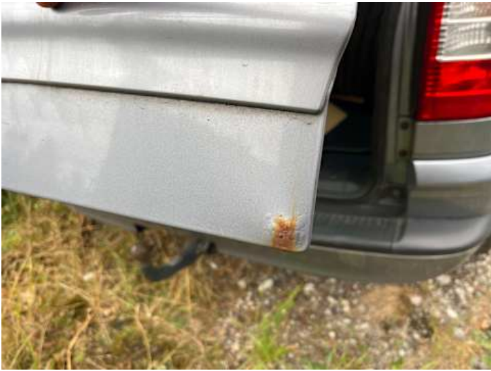
Heckklappe (Lackschaden, Rost)
