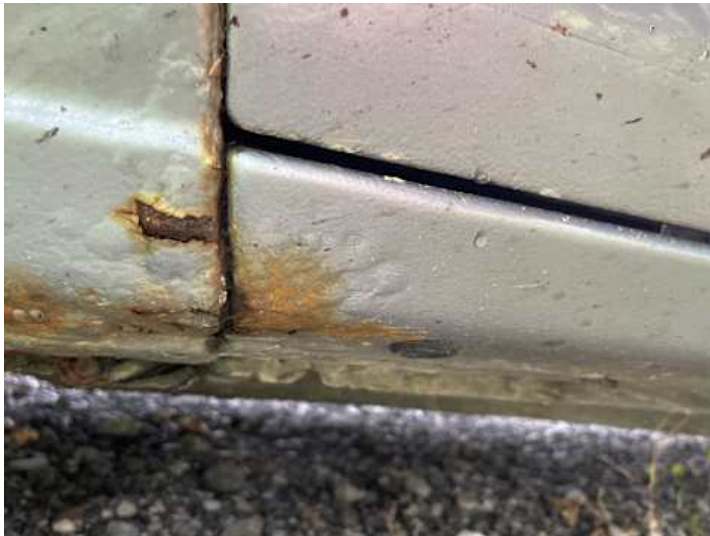
Schweller links (Lackschaden, Rost)
