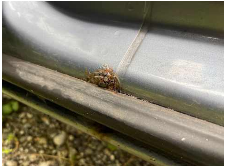
Schweller links (Lackschaden, Rost)
