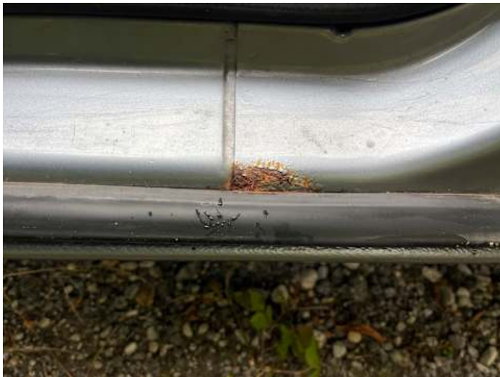
Schweller links (Lackschaden, Rost)
