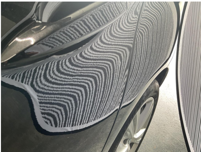
Tür hinten links - Delle entfernen
