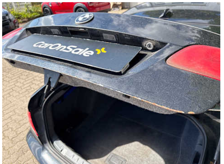
Heckklappe (Lackschaden, Rost)
