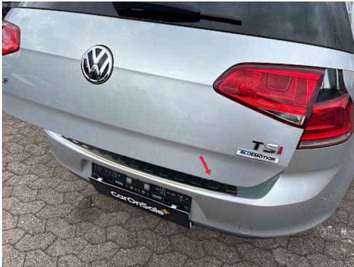
Heckklappe (Lackschaden, Rost)
