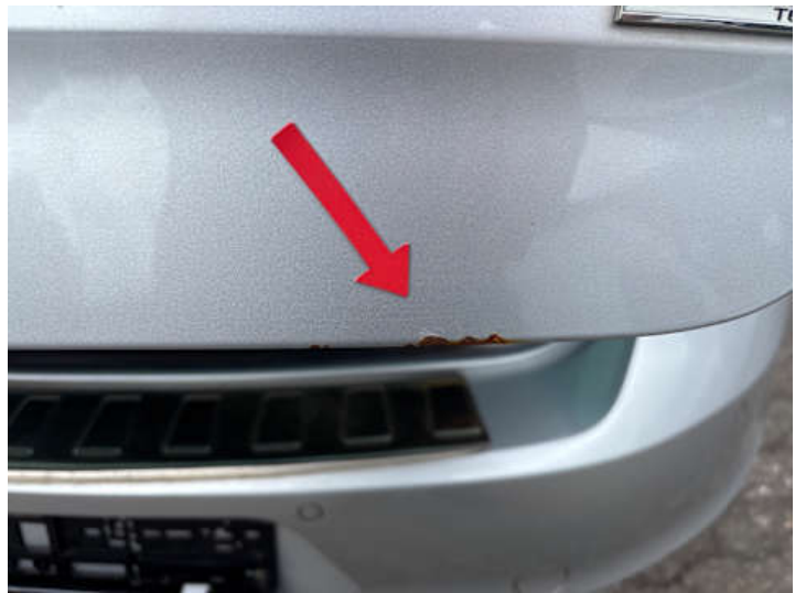
Heckklappe (Lackschaden, Rost)
