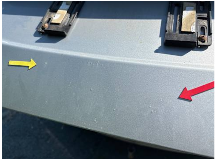
Heckklappe (Lackschaden, Rost)
