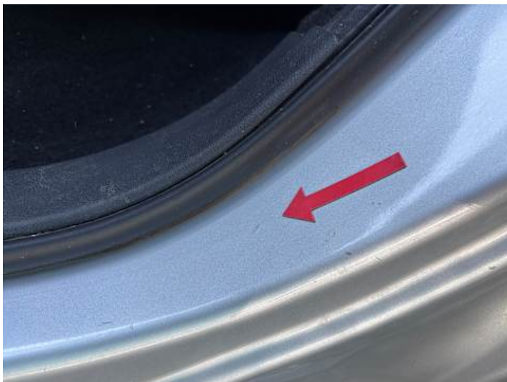
Türe hinten links (Lackschaden, Rost)
