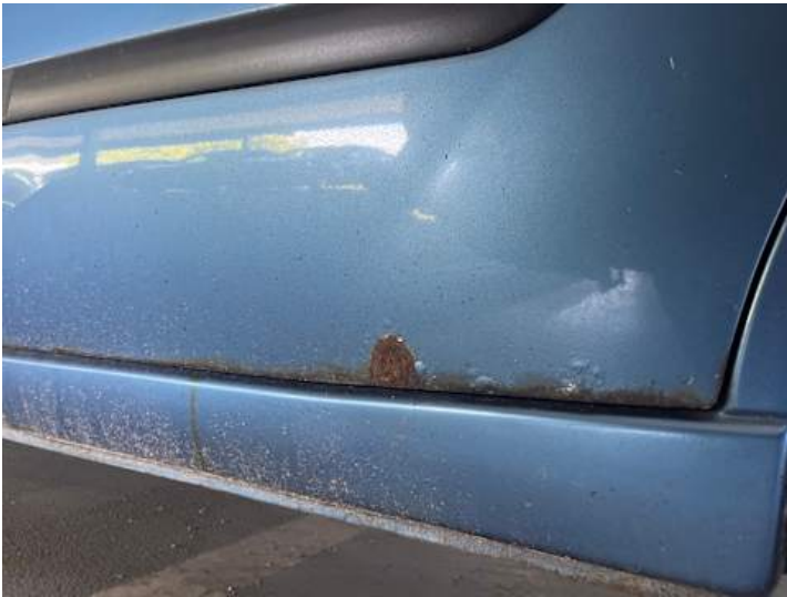
Türe hinten links (Lackschaden, Rost)
