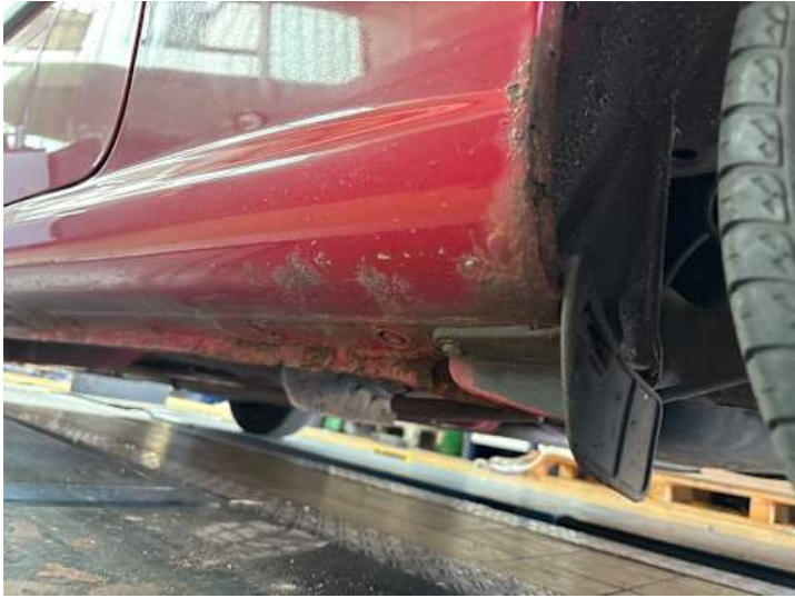
Schweller links (Lackschaden, Rost)
