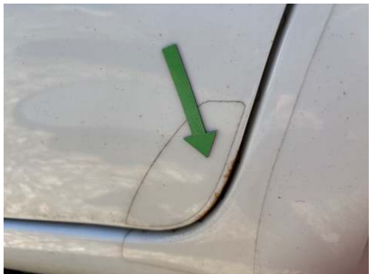
Türe hinten links (Delle, Rost)
