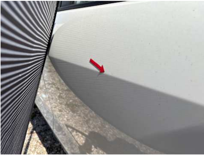
Türe hinten links (Delle, Rost)
