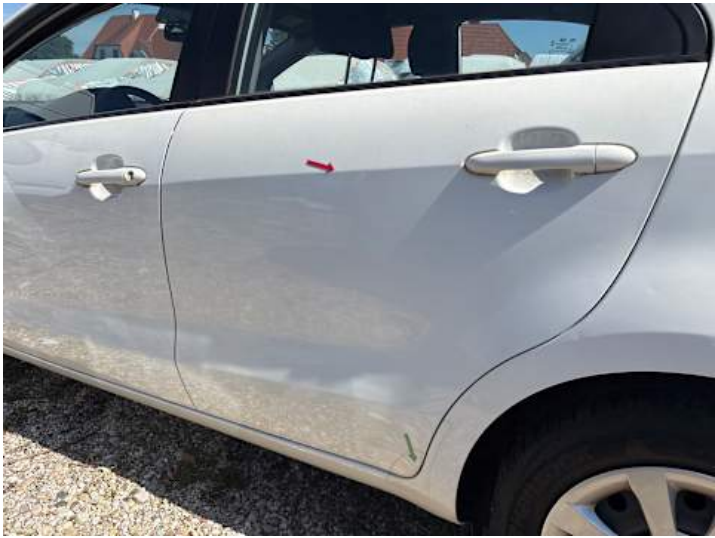
Türe hinten links (Delle, Rost)
