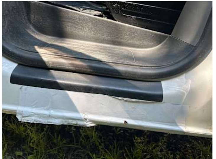
Schweller links (Riss/Bruch, Rost)
