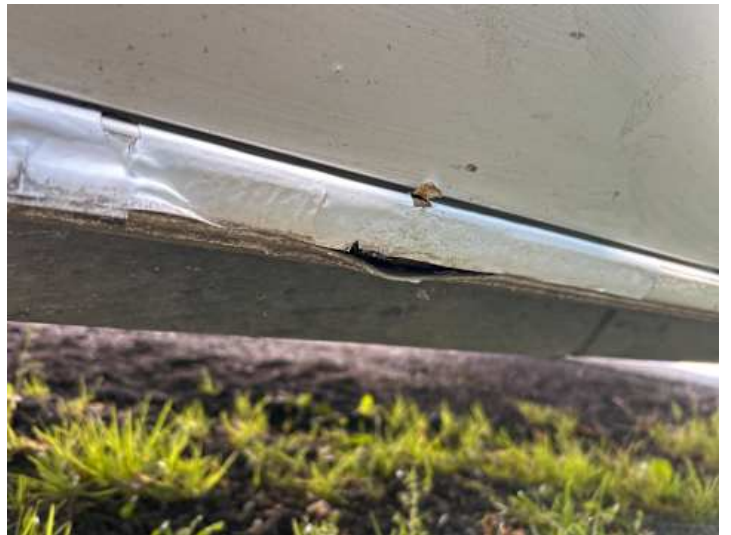
Schweller links (Riss/Bruch, Rost)
