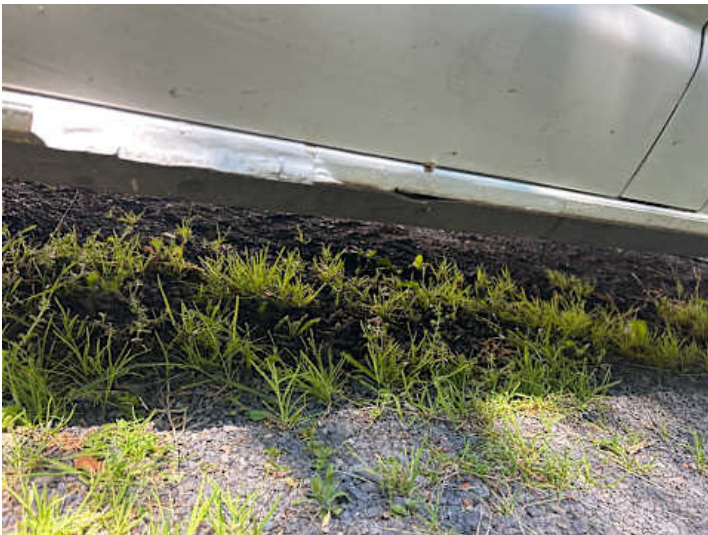
Schweller links (Riss/Bruch, Rost)
