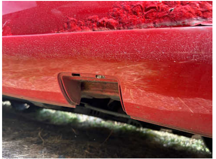
Schweller links (Riss/Bruch, Rost)
