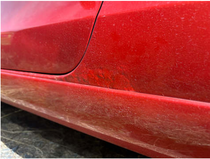
Schweller links (Riss/Bruch, Rost)
