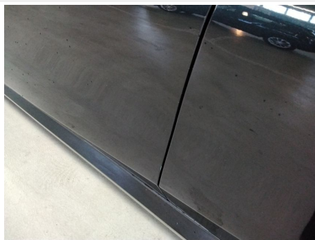
Tür / Vorne Links / Kratzer
