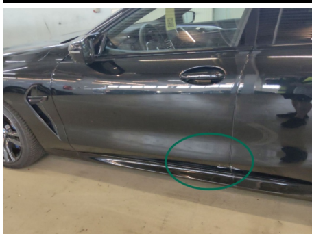
Tür / Vorne Links / Kratzer
