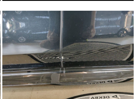
Tür / Hinten Links / Kratzer
