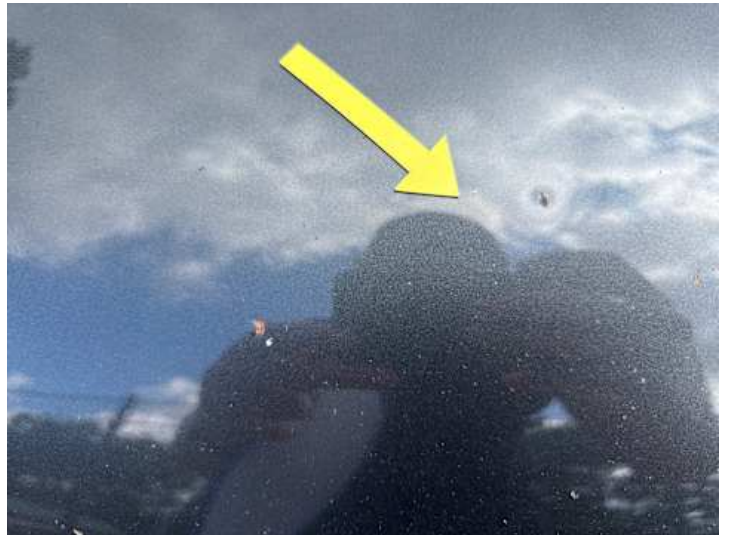
Motorhaube (Delle, Rost)
