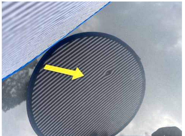
Motorhaube (Delle, Rost)
