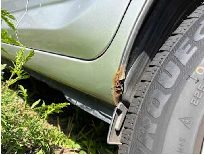
Schweller links (Lackschaden, Rost)
