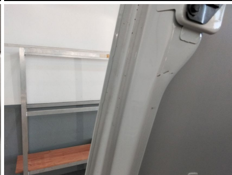
Heckklappe / Kofferraumtür / Innenraum Hinten Links / Delle
