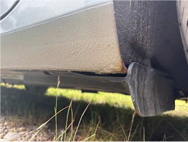
Schweller links (Lackschaden, Rost)
