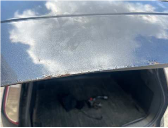
Heckklappe (Lackschaden, Rost)
