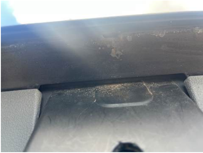
Heckklappe (Lackschaden, Rost)
