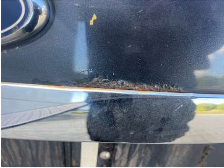
Heckklappe (Lackschaden, Rost)
