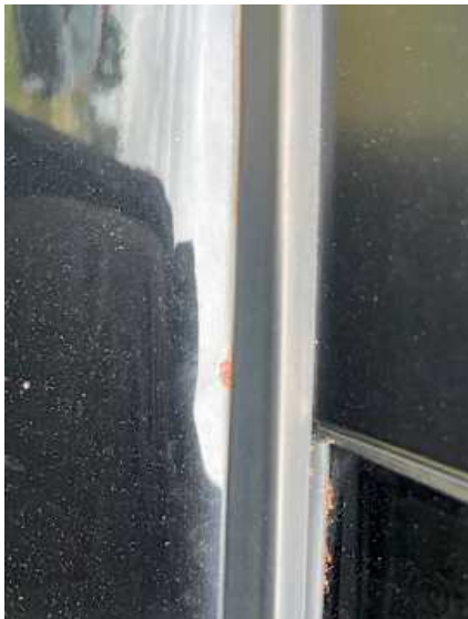
Türe hinten links (Lackschaden, Rost)
