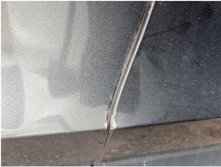
Türe hinten links (Lackschaden, Rost)
