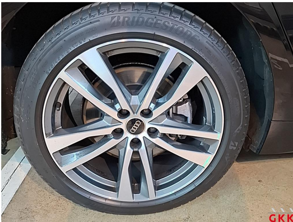
Picture 22 LM wheel, rear right, scratched, replace
