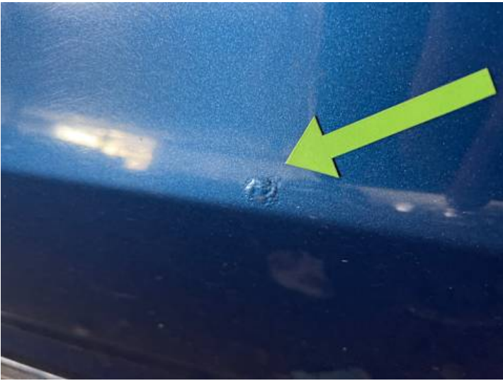
Türe hinten links (Lackschaden, Rost)
