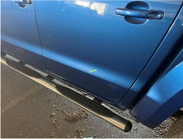
Türe hinten links (Lackschaden, Rost)
