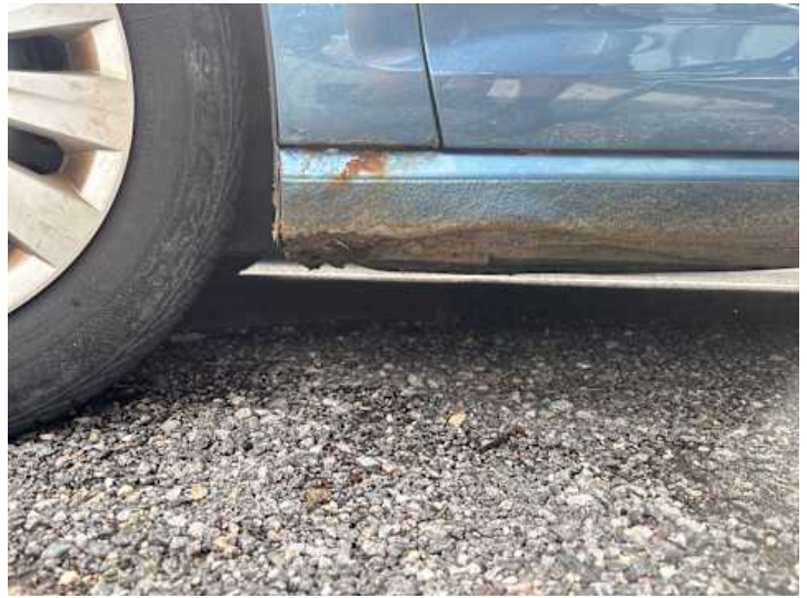
Schweller links (Lackschaden, Rost)
