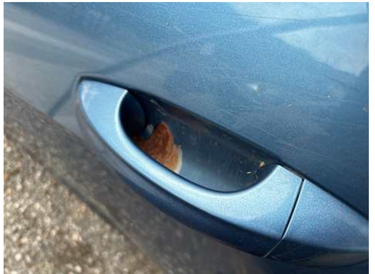
Türe hinten links (Lackschaden, Rost)
