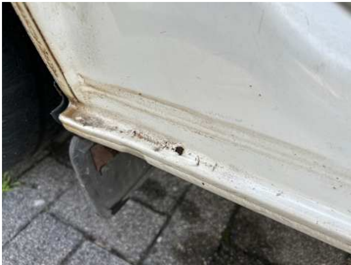
Schweller links (Lackschaden, Rost)
