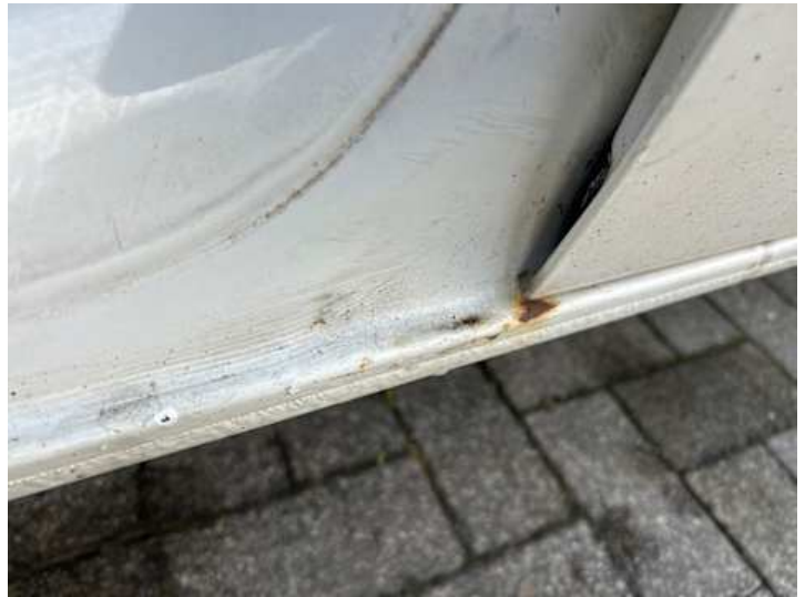
Schweller links (Lackschaden, Rost)
