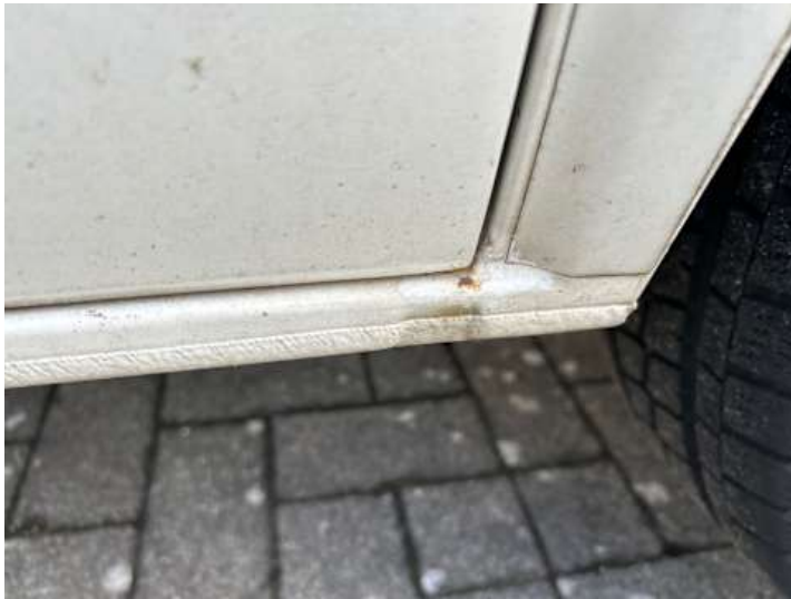
Schweller links (Lackschaden, Rost)
