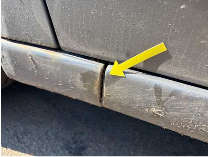
Schweller links (Lackschaden, Rost)
