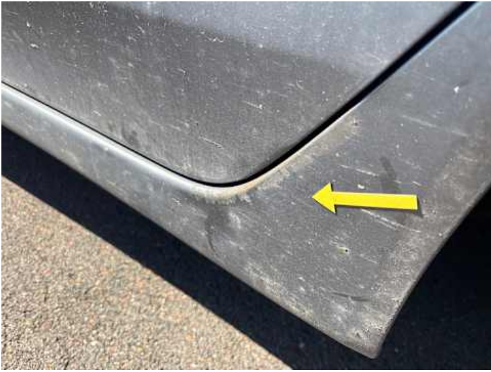
Schweller links (Lackschaden, Rost)
