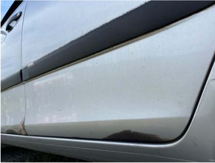
Türe hinten links (Delle, Rost)
