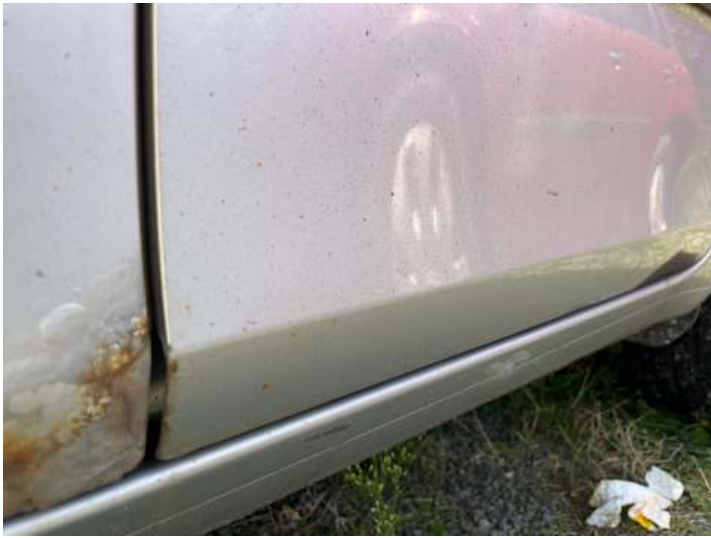
Türe hinten links (Delle, Rost)
