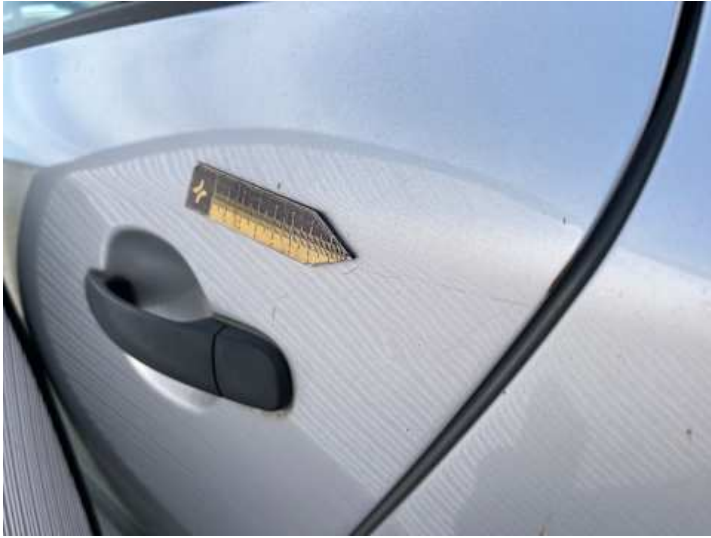
Türe hinten links (Delle, Rost)
