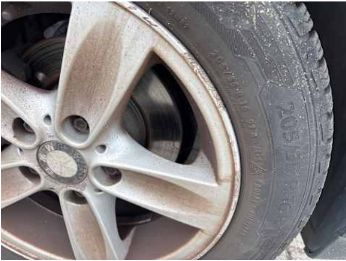
Rad (vehicle.damage-label.porous, Kerben, Rost)
