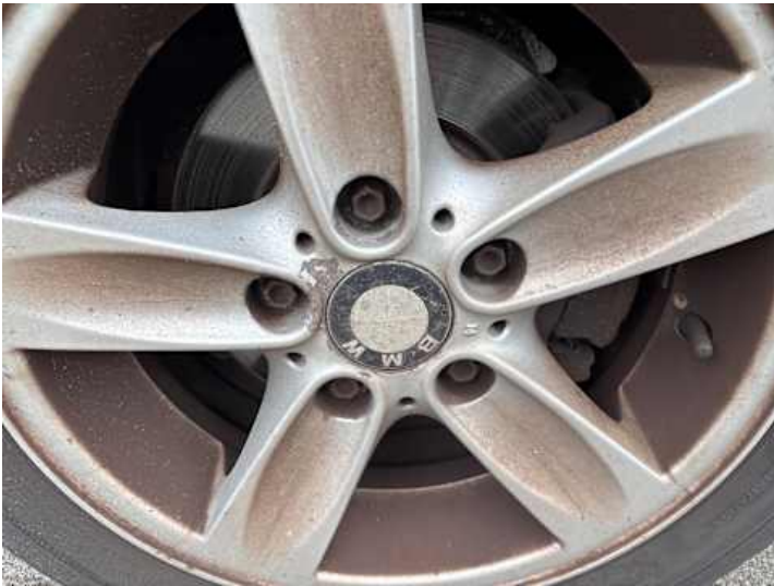
Rad (vehicle.damage-label.porous, Kerben, Rost)
