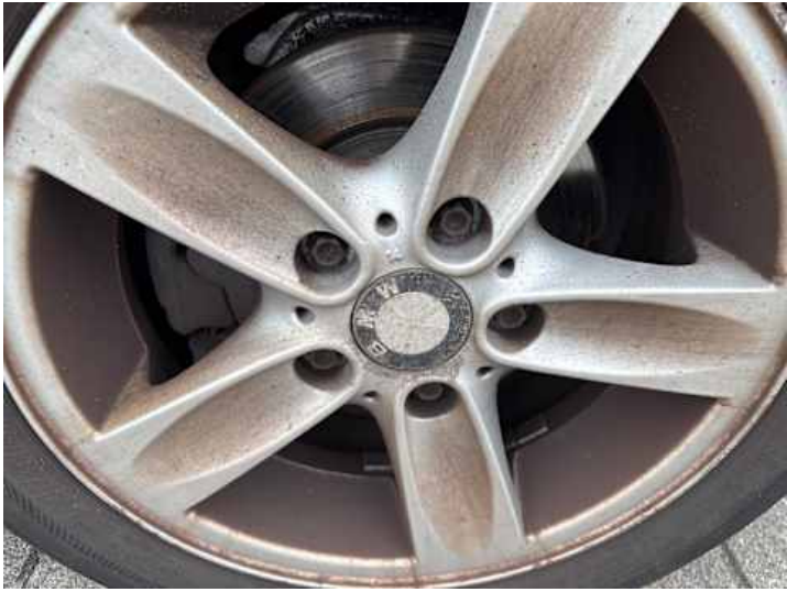
Rad (vehicle.damage-label.porous, Kerben, Rost)
