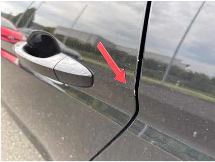
Türe hinten links (Lackschaden, Rost)
