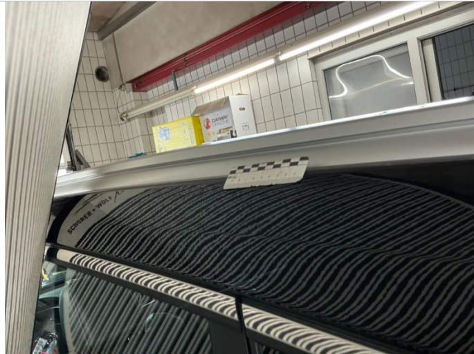
Dachholm links Dellen.
