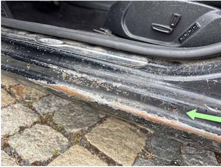
Schweller links (Lackschaden, Rost)
